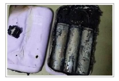
The charge control circuit has been burned here in this faulty power bank when it was supposed to save the product from over charging. The very thing that is supposed to save customers from harm from overcharged batteries was too cheaply made... maybe 50 cents worth of higher specification electronics would have avoided this. On cheap power banks, 50 cents can make all the difference.
