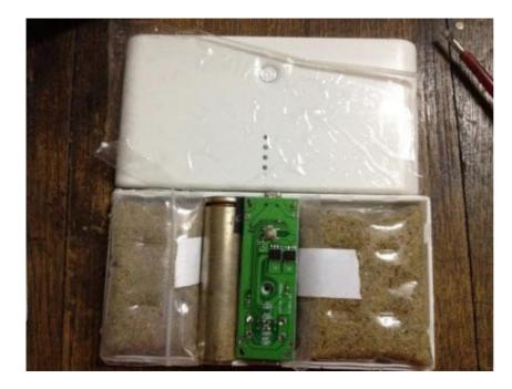
This is an example of how far some companies are willing to go to make more profit. This charger should have 6 batteries..... instead it has one battery and two bags of sand. Feels correct weight wise but works badly.
