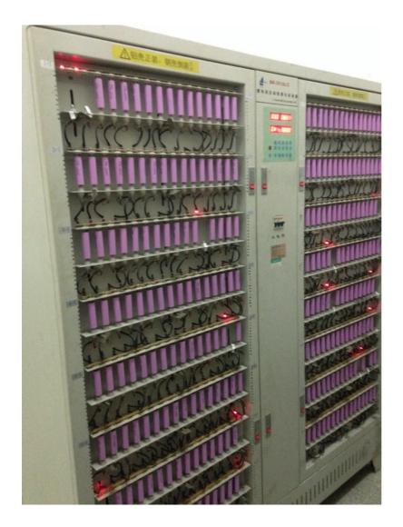
Age testing machine left, and below a final charge before shipping.
