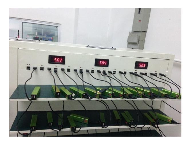
From many conversations with distributors we understand that a lot of chargers supplied in the USA today are failing after one or two charges and do not not hold a charge. This could be avoided, by companies wanting to supply the safest and most reliable product, by buying Grade A batteries and then age testing them..... of course, manufactures cutting corners will not do this.
